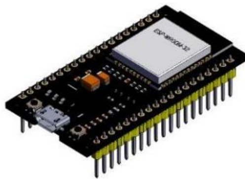
Gambar 2. 3 Gambar ESP32 (Mardianto, 2023)
