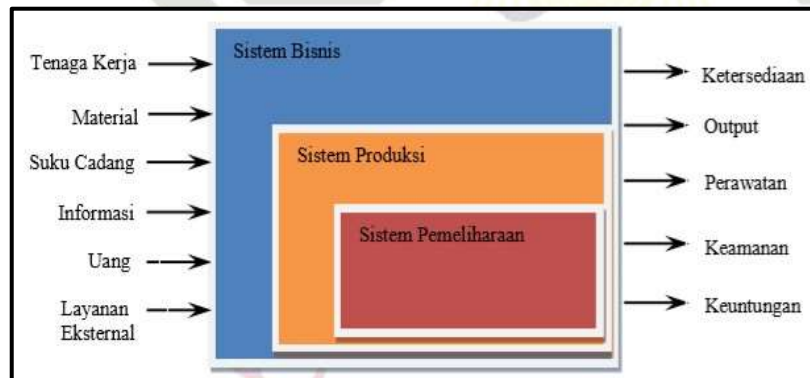
Gambar 2.1 Model Input-Output Proses Maintenance (Sumber: Pranowo, 2019)
