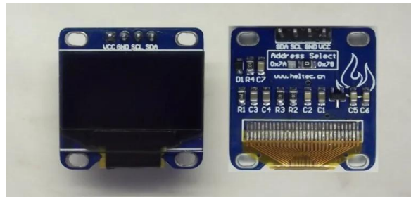
Gambar 2. 9 OLED 0,96 inci 128x64
