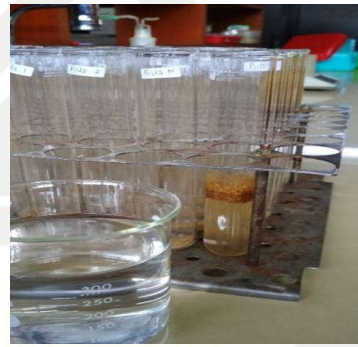
Gambar 9. Penambahan Larutan Buffer McDougall sebanyak 40 mL
