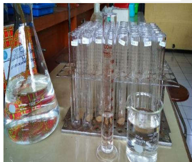
Gambar 10. Penambahan Larutan Buffer McDougall sebanyak 40 mL
