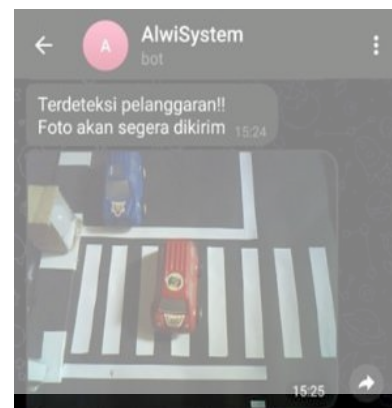
Figure 7. Notification of esp32 cam result to Telegram
