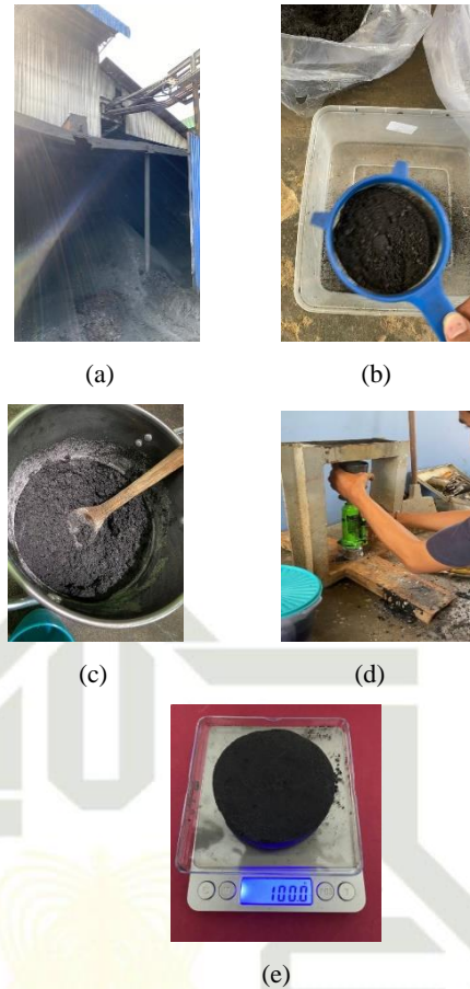
Figure 3. Making Bio-briquettes (a) Boiler Ash, (b) Boiler Ash Filtering, (c) Boiler Ash Mixing, (d) Bio-briquette Printing, and (e) Bio-briquette Results
