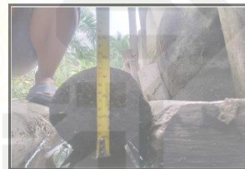
Gambar 4 diameter kayu pancang
