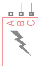
Gambar 2.31 Three Phase Fault [34]
