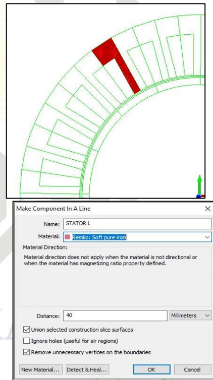
Figure 3. Making Components on the Stator and Rotor with Material Remko: Soft Pure Iron.
