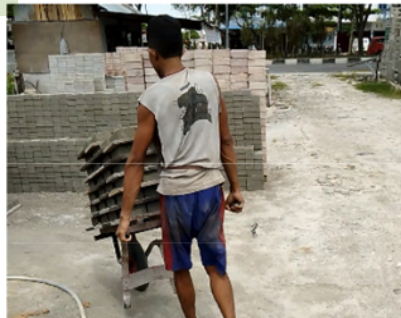
Figure 2 Workers transporting paving blocks ready for printing to drying places (see online version for colours)
