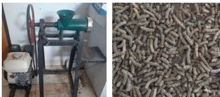
Photo 2. The machine for making pellets from oil palm frond and Indigofera foliage
