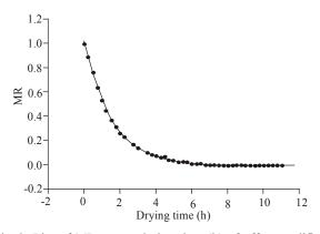
Fig. 3: Plot of MR versus drying time (h) of offset modified page (new model) model at 20% RH and  $T = 50^{\circ}C$
