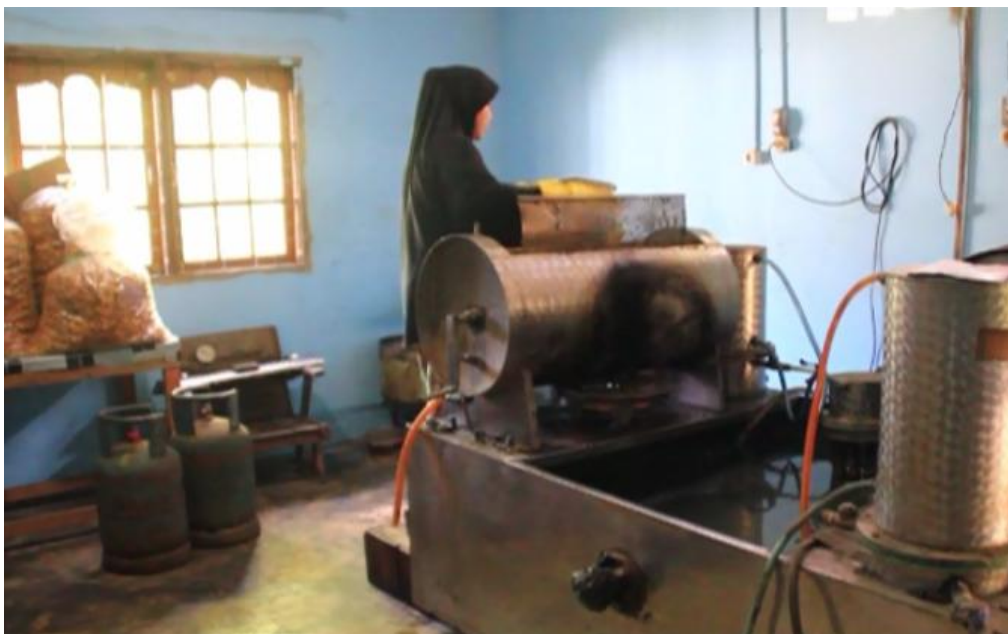
Figure 1.2 The Production of Pineapple Chips using Vacuum Frying Machine in Kualu Nenas
