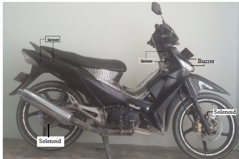
Figure 12 Position of Sensor and Solenoid crossbeam
