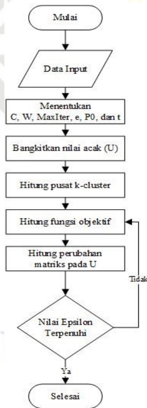
Gambar 2.1. Flowchart Algoritma Fuzzy C-Means
