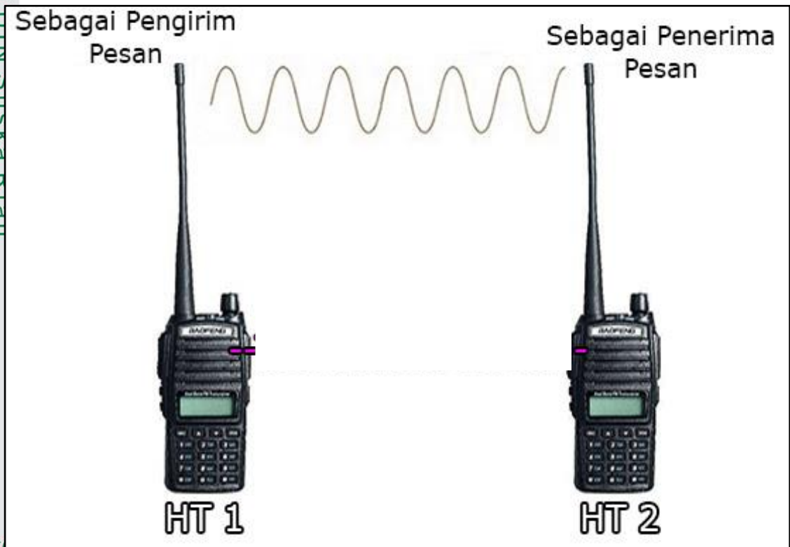
Gambar 2.5 Skema cara kerja Handy Talky (HT) [21].
