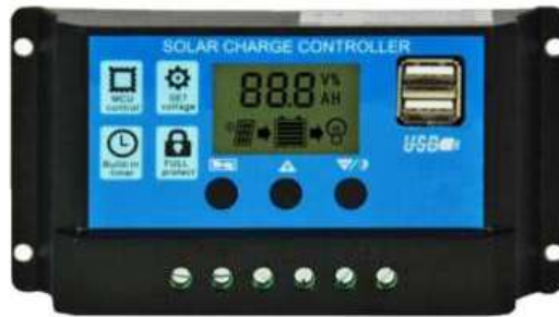
Gambar 2. 13 Solar Charger Controller
