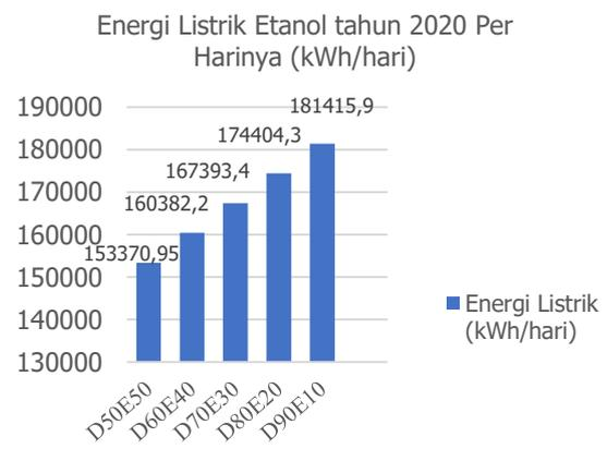
Gambar 3. Grafik Energi Listrik Etanol D50E50, D60E40, D70E30, D80E20, dan D90E10
