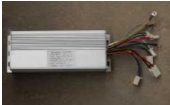
Gambar 2. 7 Controller Motor Brushless DC
