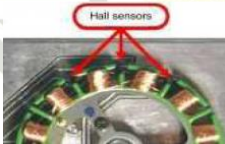
Gambar 2. 6 Sensor Hall Motor Brushless DC
