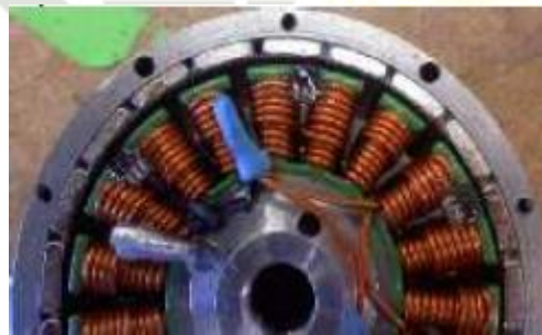
Gambar 2. 5 Stator Motor Brushless DC
