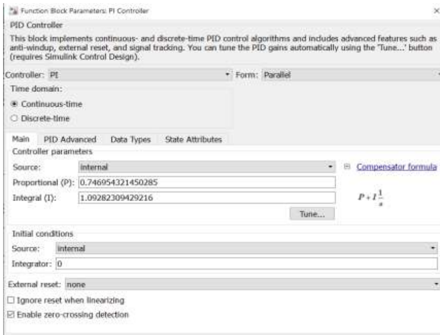
Gambar 3. 5 Tampilan blok PI Controller
