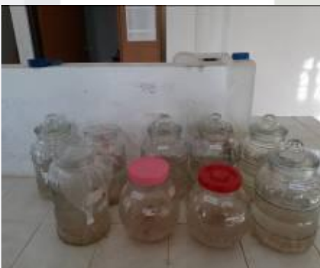
Proses perendaman HCl selama 20 jam
