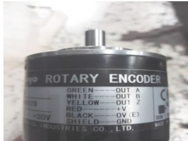
Gambar 2. 7 Rotary encoder (Sumber: PT. Asia Forestama Raya 2018)
