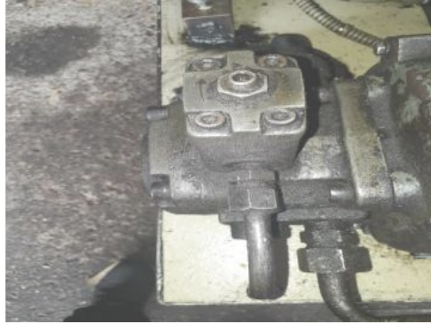
Gambar 2. 11 Pump hydraulic (Sumber: PT. Asia Forestama Raya 2018)
