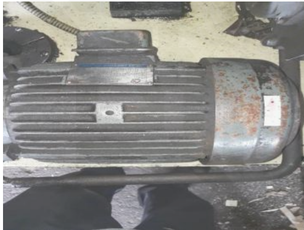
Gambar 2. 10 Motor pump hydraulic (Sumber: PT. Asia Forestama Raya 2018)
