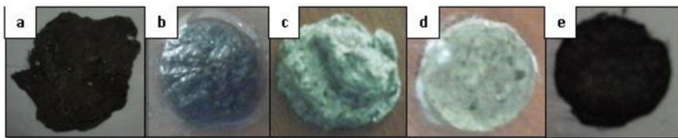
Figure 2. The sample for each step in preparation process: a) a spider web once collected, (b) after washing, (c) after drying, (d) after compression, (e) after carbonization.
