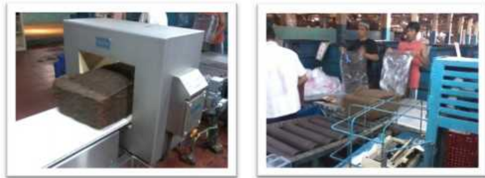
(a) Metal Detector , (b) Pengemasan Gambar 4.10 Proses Pengemasan Bandela SIR 20
