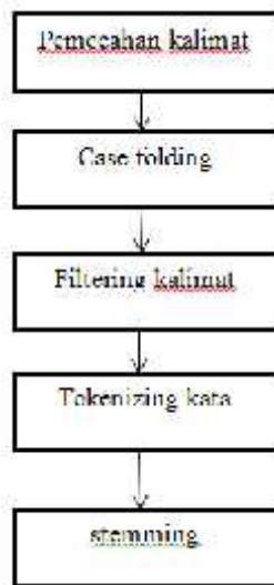
Gambar 2.1 Proses text preprocessing
