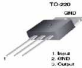
Gambar 2.17. IC Regulator LM7805 (Sumber: Bishop, 2004)
