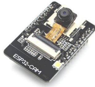
Gambar 2.7 Modul ESP32 CAM Wi-Fi [14]
