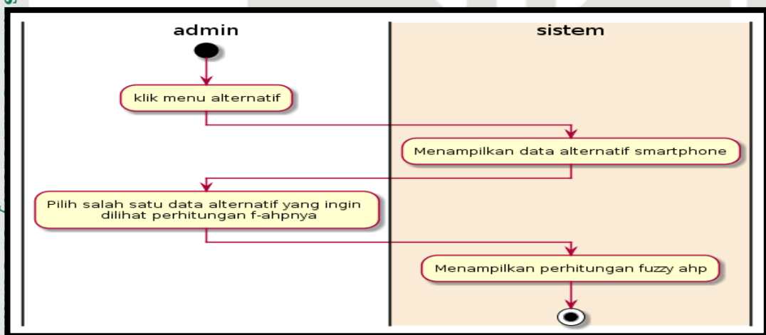
Gambar 4. 9 Activity Diagram Perhitungan Alternatif Smartphone
