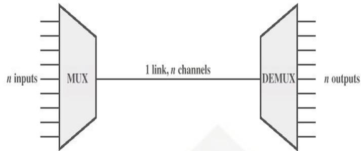
Gambar 2.8. Prinsip Dasar *Multiplexing*
