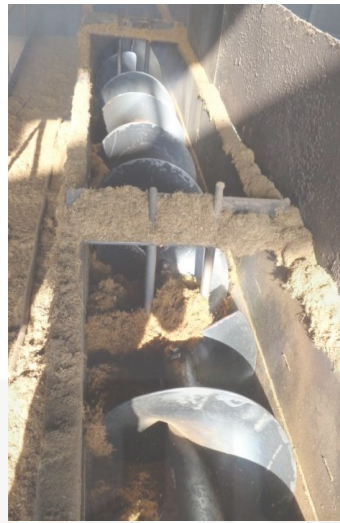
Gambar 2.5. Distributor Conveyor (Sumber: Effendy 2013)
