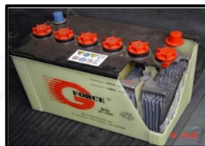
Gambar 2.17 Starting Battery (Sumber: Nasution, 2016)
