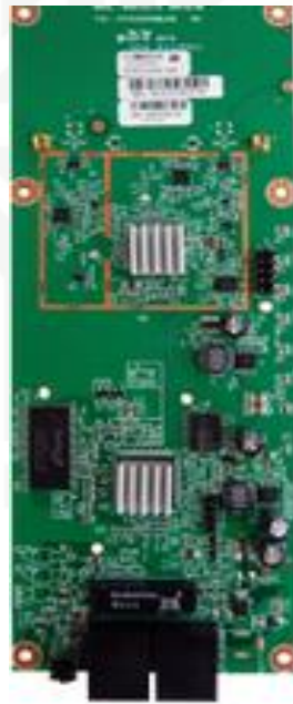
Gambar 3.14 radio board ALFA N5 PCBA
