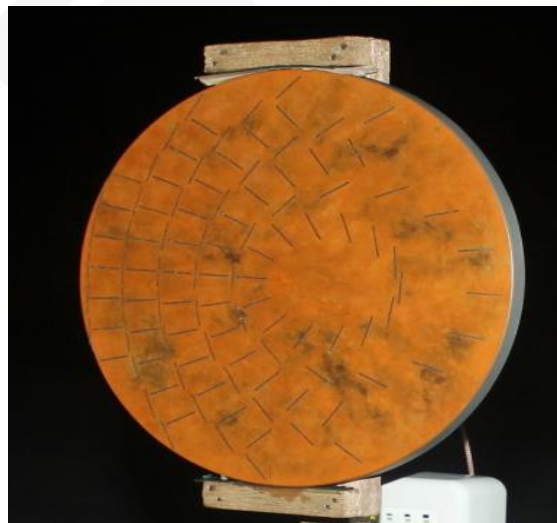
Gambar 2.1. Antena Radial Line Slot Array (Sumber : Awaludin Jamil, 2015)
