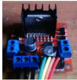
**Gambar 2.8 Modul driver motor L298**
