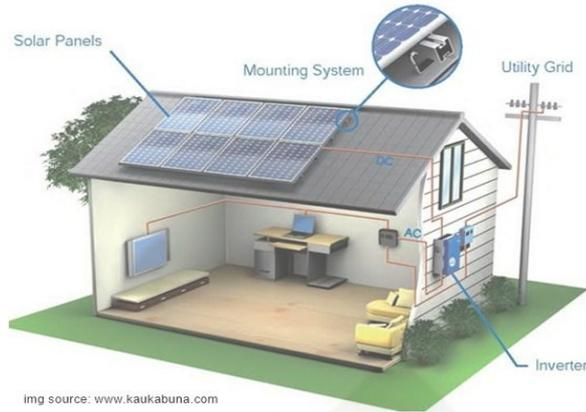
Gambar 2.5 Prinsip Kerja PLTS *On-Grid*
