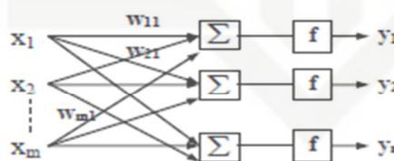
Gambar 2.3. Model JST Satu Lapisan (Widagda, 2012)
