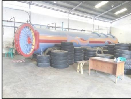
Gambar 4.12 Mesin Chamber
