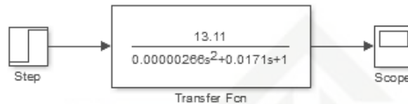
Gambar 3.2. Blok diagram simulink sistem Motor BLDC
