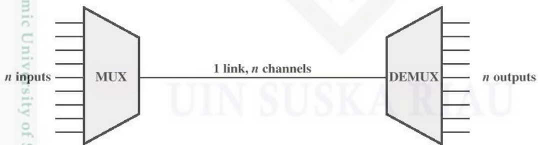
Gambar 2.7. Prinsip Dasar Sistem WDM (Sumber: Sri Mayati, 2015)
