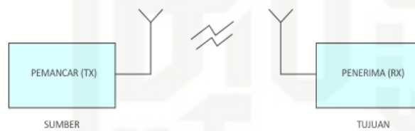
Gambar 2.3. Diagram Blok Komunikasi Radio (Sutoyo, dkk, 2013) [23]
