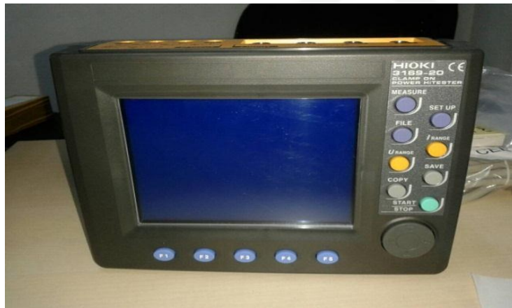
Gambar 3.3 Power Analyzer/Data Taker
